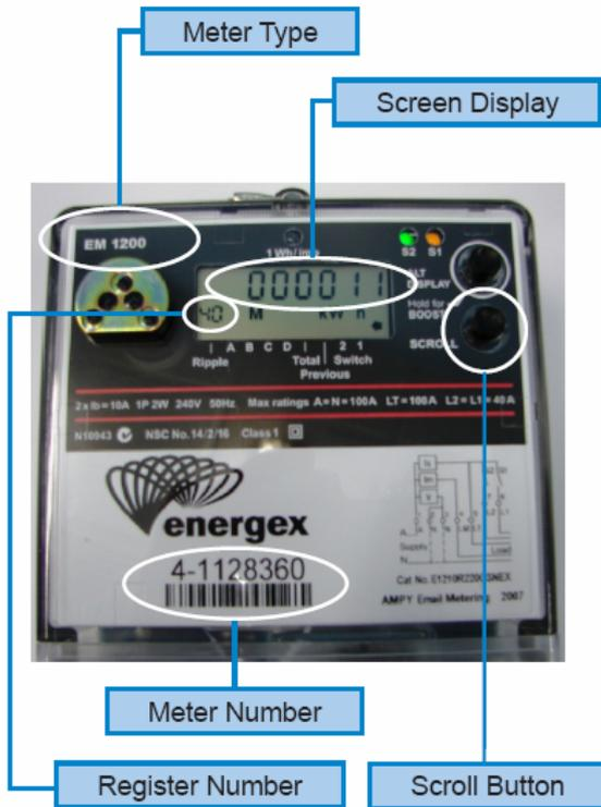
These electronic meters are able to provide more than one reading, for example Tariff 11 or Tariff 12 (light and power consumption) and 9900 solar feed in. The EM1200/10 series meters can also display super economy tariff 31 or economy tariff 33 (controlled supply) consumption.
